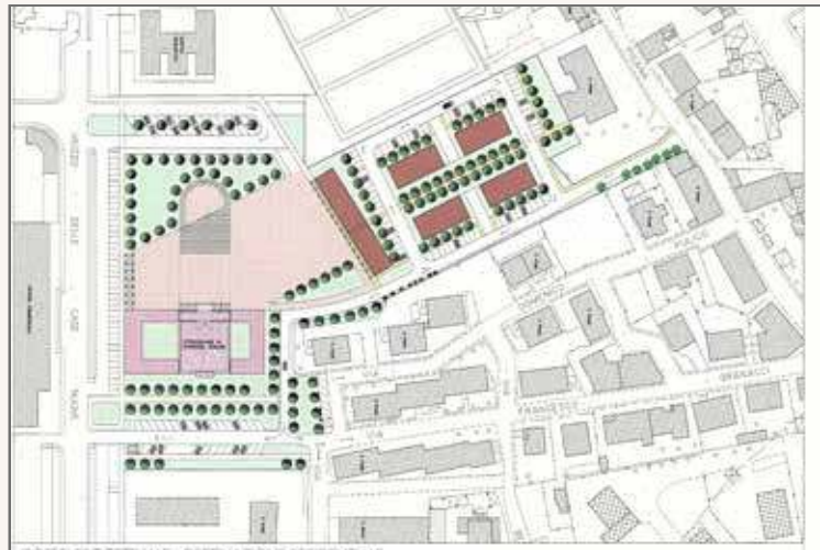
3) Site plan of a project proposal that involves the integration of the new residential development with the existing public green area
